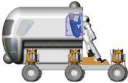
Figure 54: Suitport illustration from (Gernhard et al, 2008) reduces loss of air when exiting or entering the rover and greatly reduces the dust problem.
