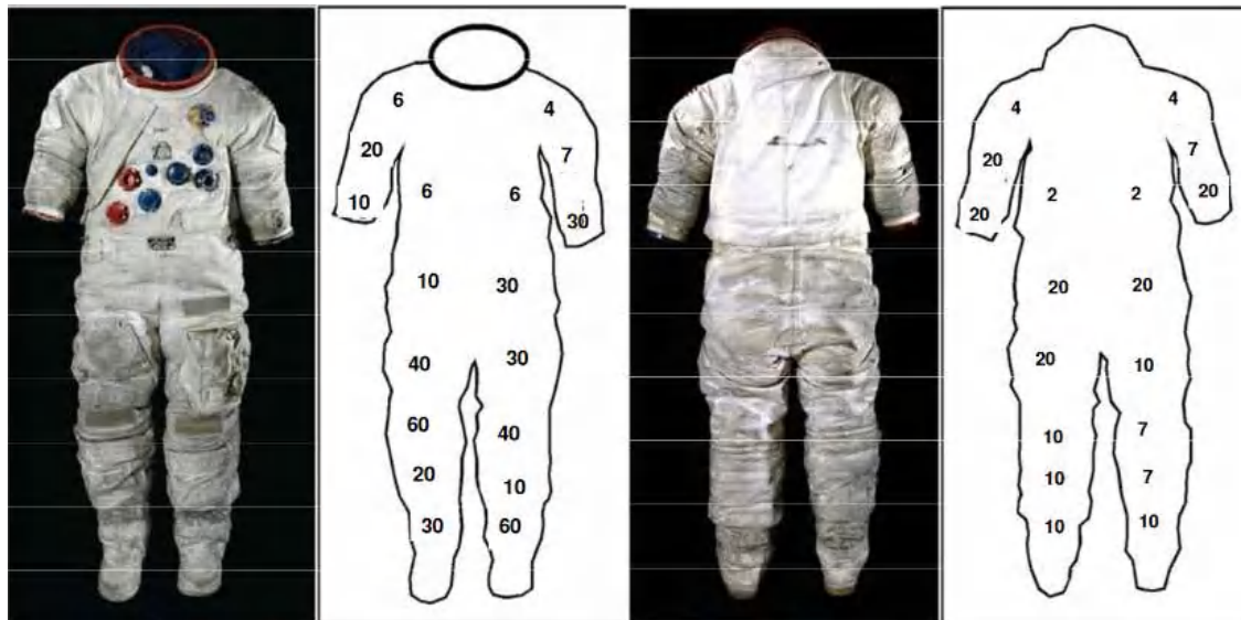
Figure 69: Concentrations of titanium (in units of 100 ppm) in the suit fabric for Jack Schmitt's suit for Apollo 17. This seems to be a good tracer of the lunar dust.
