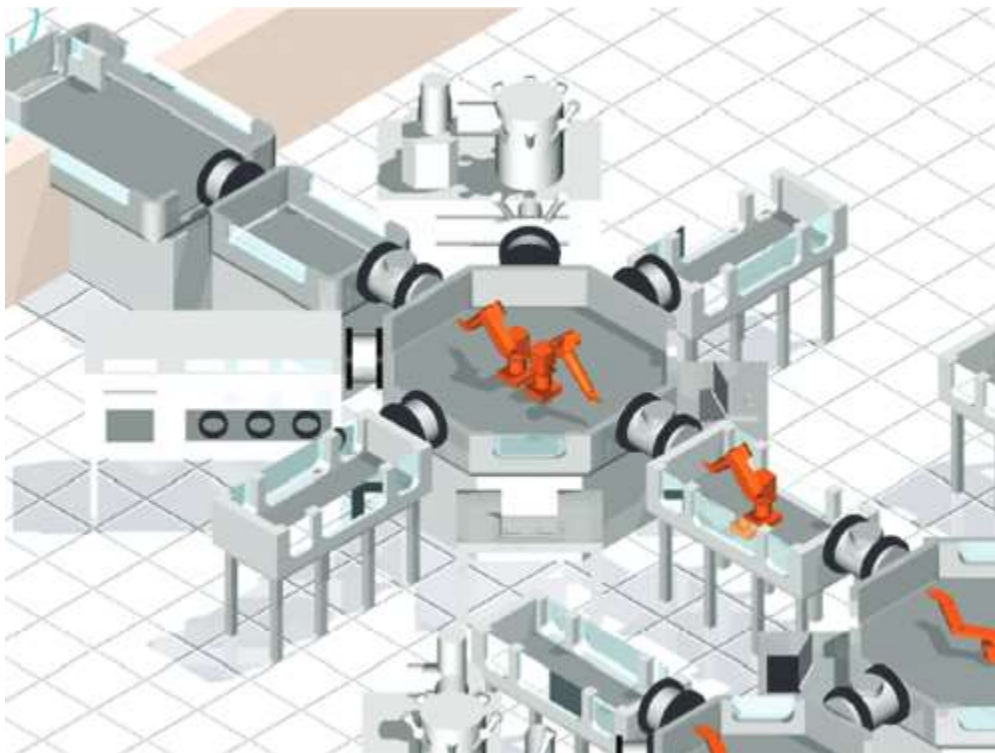
Figure 16: the LAS fully robotic floor plan for a Mars sample receiving facility.
