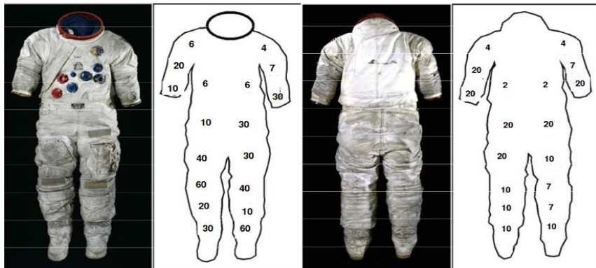
Figure 69: Concentrations of titanium (in units of 100 ppm) in the suit fabric for Jack Schmitt's suit for Apollo 17. This seems to be a good tracer of the lunar dust.
