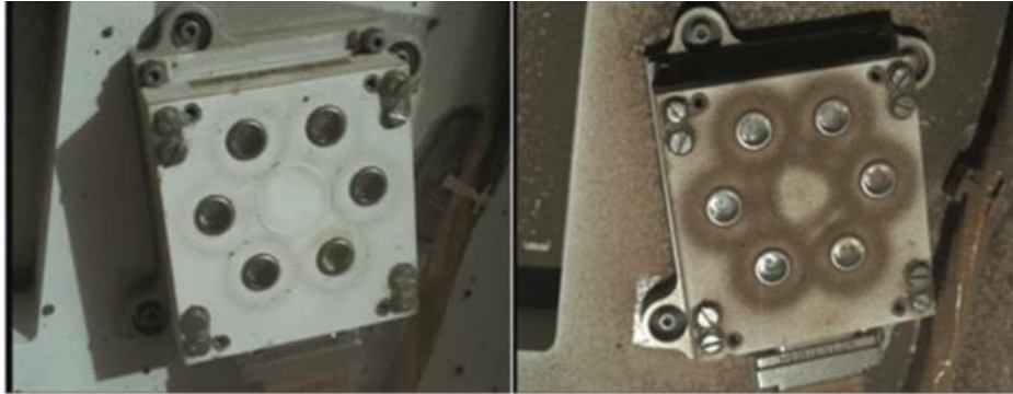
Figure 43: MAHLI images of the REMS UV Sensor on sols 36 (left) and 1314 (right) of the MSL mission. The circular patterns are caused by circular magnets around the UV sensors which attract the dust. The magnets help to keep the sensors free of dust.
