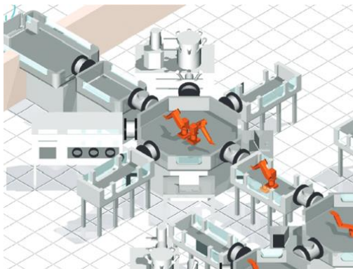
Figure 16: the LAS fully robotic floor plan for a Mars sample receiving facility.
